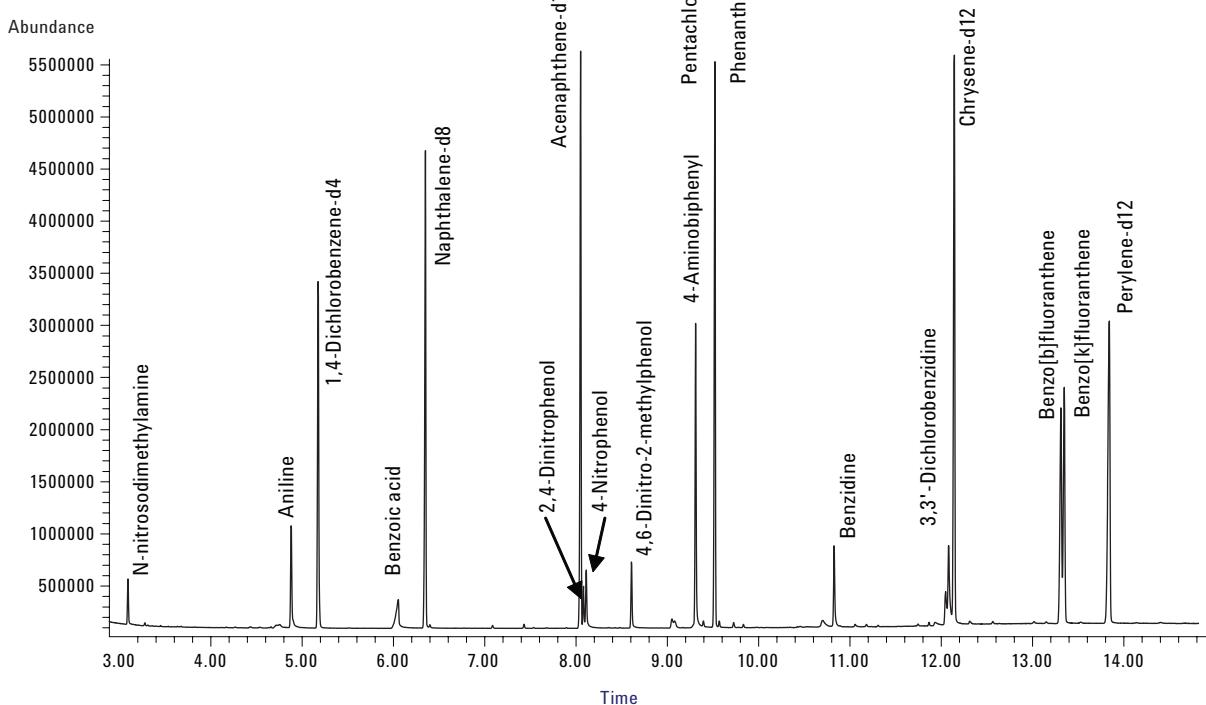
**Figure 4. Reference chromatogram for Fast 8270 method.**
