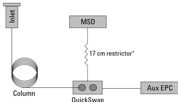
\*QuickSwap restrictor, P, and T are selected for desired flow to MSD, usually the maximum flow that the current application requires.
