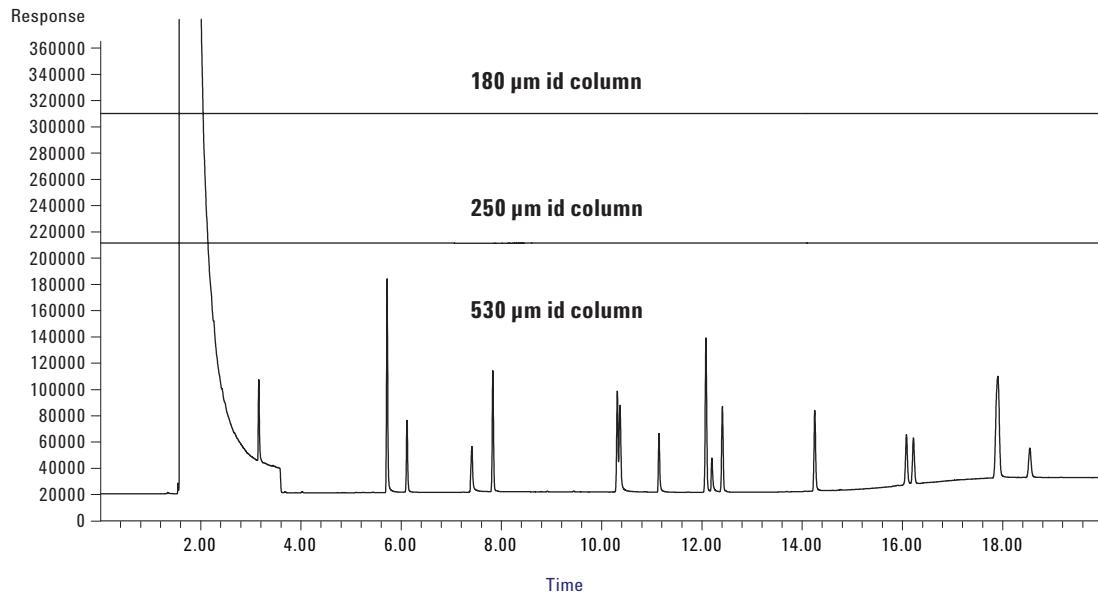
**Figure 8.** FID vent signal for three columns under optimal flow conditions. Only the 530-μm id column has a flow that exceeds the 1 mL/min flow to the MSD.
