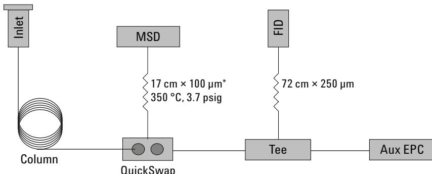
\*In this example, the restrictor, transfer line temperature, and QuickSwap pressure were chosen to allow approximately 1 mL/min flow to the MSD—corresponding to its optimal performance regime.
