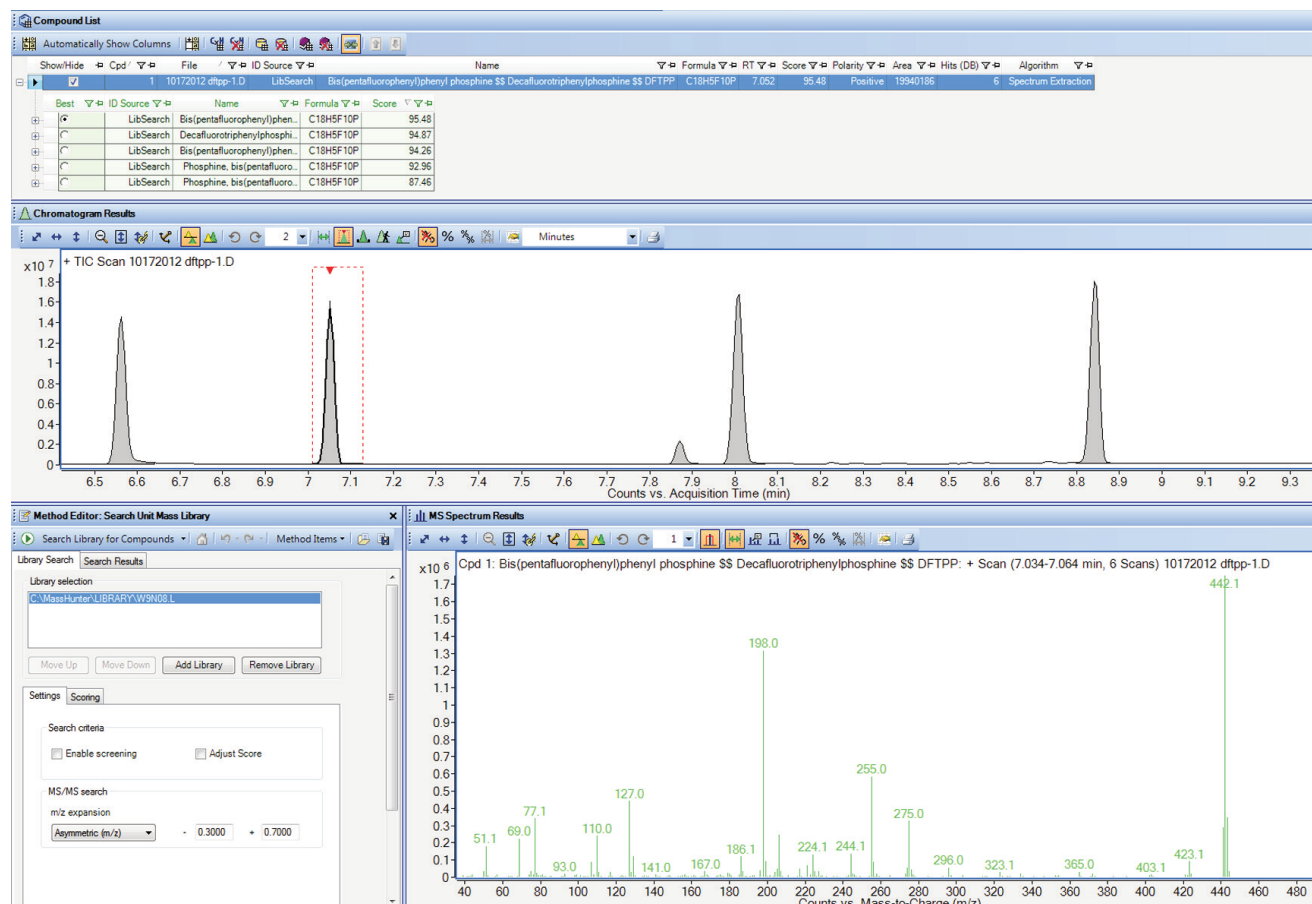
Figure 2. Evaluation of the instrument performance by spectral matching DFTPP to the NIST library.
