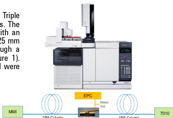
Figure 1. Column Configuration for Optimal MRM Application.
