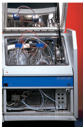
Figure 5. Agilent PL-GPC 220 integrated solvent delivery system
