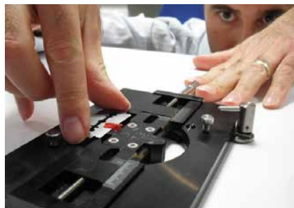
Step 3. Cross-section sample with razor.
