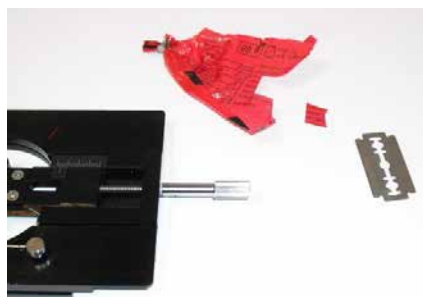
Step 1. Cut a small piece of sample.
