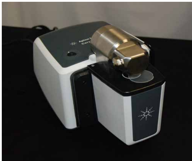
Figure 1. The Agilent DialPath transmission cell used for polymer analysis of coupons or films
