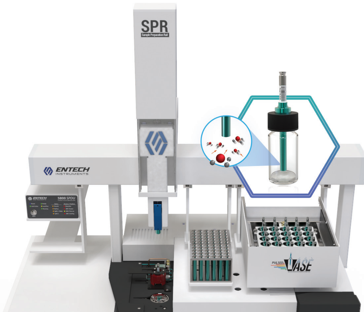
Figure 4 - A 5800 Sorbent Pen Desorption Unit (SPDU) and Entech Sample Preparation Rail (SPR) Autosampler installed onto an Agilent GCMS. After sample extraction via Pulsed VASE, the fully automated SPR transfers the Sorbent Pens from the vials in the Pulsed VASE tray to isolation sleeves prior to transferring each Sorbent Pen in sequence to the 5800 SPDU for direct thermal desorption onto the GC column.
