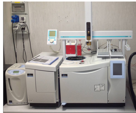
GC/MS equipped with CombiPAL XT autosampler and automated HS-SPME feature.
