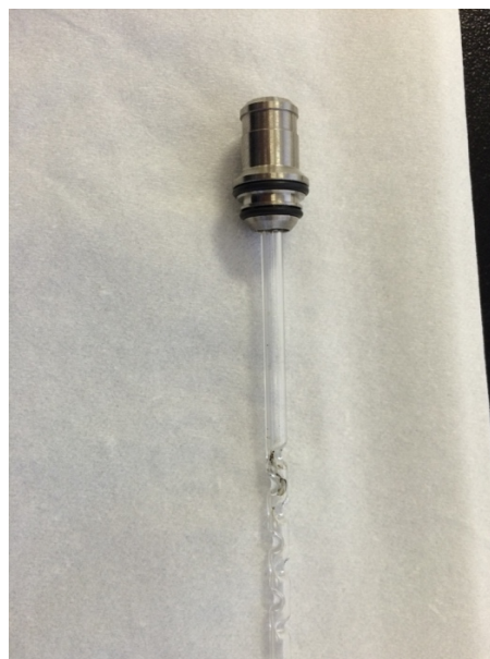
Figure 3 – Dirty liner after a few injections of the dirty QuEChERS extracts
