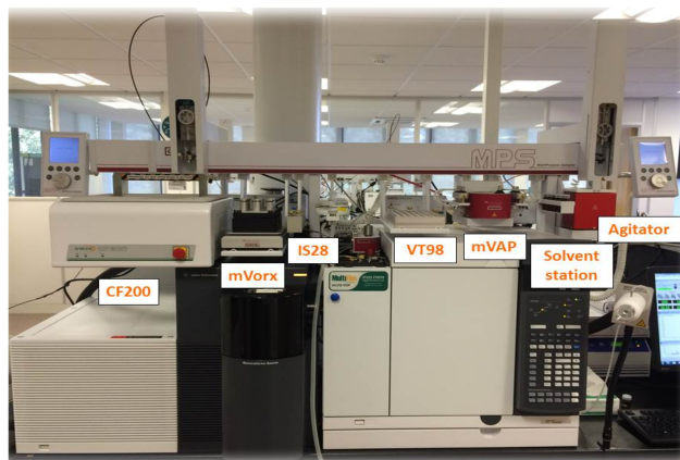
Figure 1 - Dual Head MPS xt with Centrifuge (CF-200) and Vortex (mVortex) on a GC/Q-TOF
