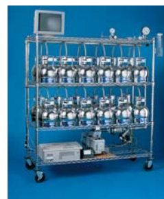
Figure 10 User-designed system for cleaning 24 six-liter canisters.
