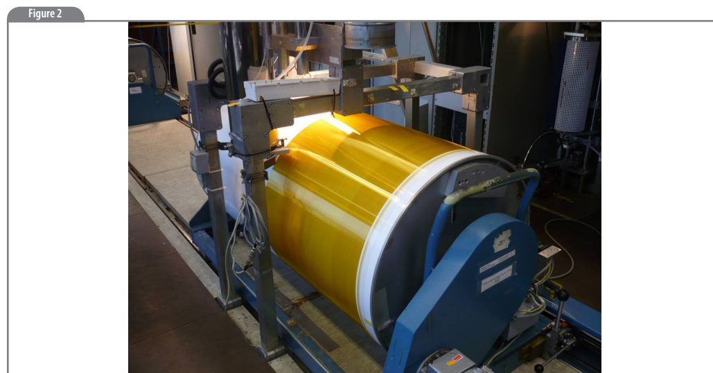
Figure 2: Wind-up drum of fused silica drawing tower of Restek: This drum can take up to 7 km of tubing.
