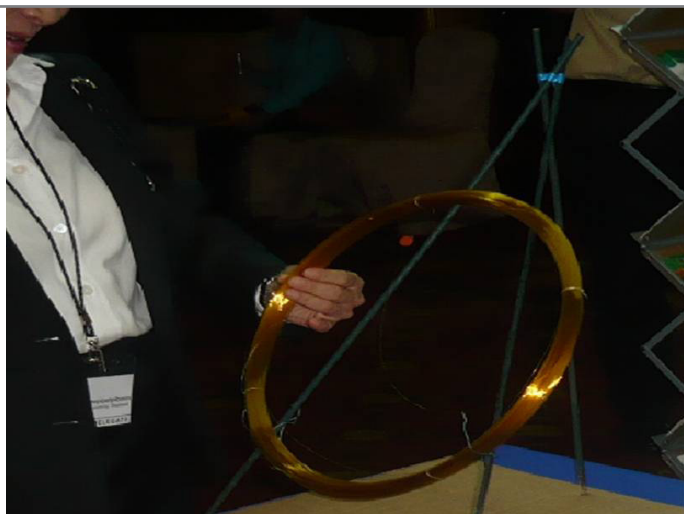
Figure 3: Example of what the world's longest fused silica column looks like.
