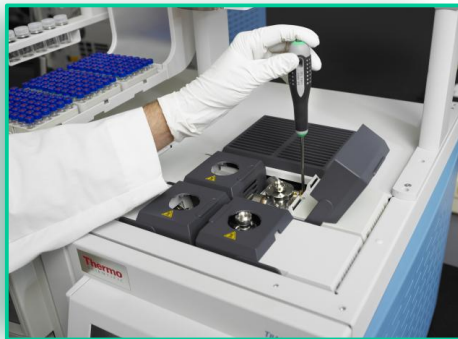
FIGURE 1. TRACE 1300 Series GC modularity with user-installable modules.
