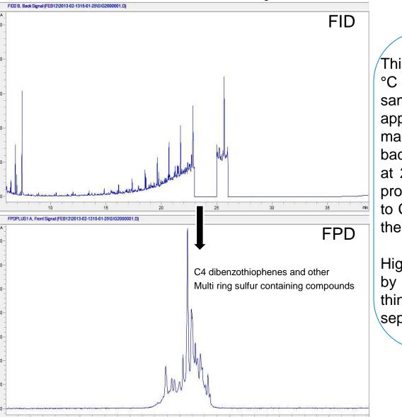
This sample has a final boiling point of 620 °C from simulated distillation data. The sample was prepared in toluene diluted approximately 20 to 1. The deans cut was made from 23 to 25 minutes, with backflush of the primary column beginning at 26 minutes. Typically, backflush will be programmed to occur at approximately C30 to C35 to protect the column set and avoid the need for long runs or bake out times.
