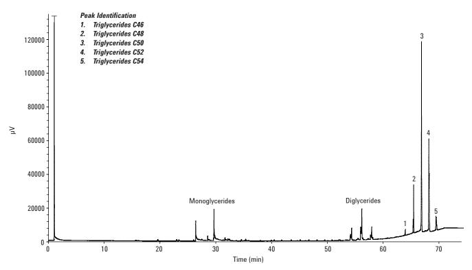
Analysis of crude palm oil using a VF-5ht UltiMetal column
