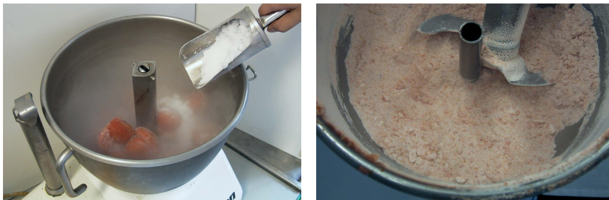
Figure 3. Left: Cryogenic sample processing using dry ice. Right: Flowable powder produced after cryogenic processing. Photographs provided by Fera, UK.
