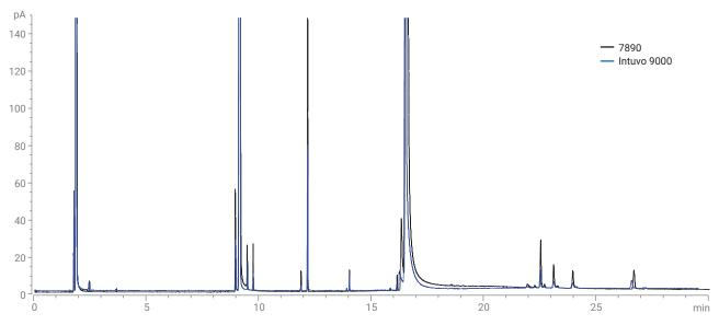
Figure 4. Sample of Flavor A liquid analyzed on a 7890 GC and Intuvo 9000 GC using a DB-HeavyWAX GC column.
