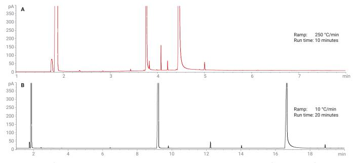
Figure 5. A sample of Flavor B e-cigarette liquid analyzed on a DB-HeavyWAX column using an Intuvo 9000 GC with a final temperature of 280 °C and ramping rates of 10 °C/min and 250 °C/min.
