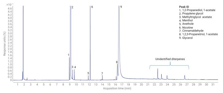
Figure 1. A sample of Flavor A e-cigarette liquid analyzed on a DB-HeavyWAX column using a 7890 GC with a final temperature of 250 °C.
