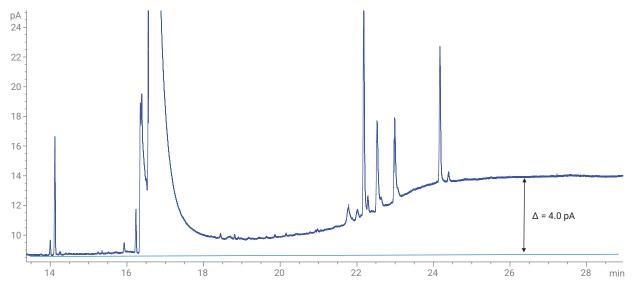
Figure 3. A sample of Flavor A e-liquid analyzed on a DB-HeavyWAX column-zoomed in on the 14-30 minutes range. Bleed only 4 pA at 280 °C.
