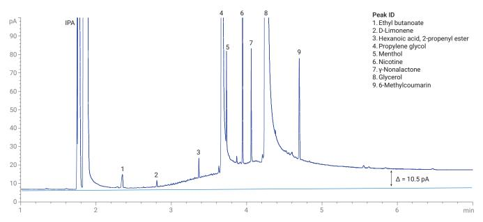
Figure 6. A sample of Flavor B e-cigarette liquid analyzed on a DB-HeavyWAX column using an Intuvo 9000 GC with a final temperature of 290 °C.
