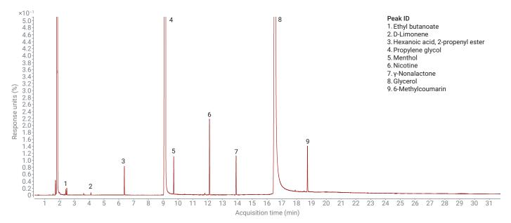
Figure 2. A sample of Flavor B e-cigarette liquid analyzed on a DB-HeavyWAX column using a 7890 GC with a final temperature of 250 °C.
