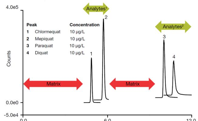
Figure 4: Column : Dionex IonPac CS21-Fast-4µm 2 x 250 mm. Injection volume: 10 µL. Flow rate: 0.3 mL/min. Eluent: 0 min – 3.0 mM MSA, 3.6 min – 3.0 mM MSA, 6.0 min – 22.0 mM MSA, 15 min – 25 mM MSA. SRM transitions as shown in Table 4.
