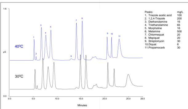
Figure 2: Column: Dionex IonPac CS17 2 x 250 mm. Injection volume: 2 µL. Flow rate: 0.4 mL/min. Eluent: 0 min – 2 mM MSA, 9.3 min – 2mM MSA, 16 min – 10 mM MSA, 22 min – 60 mM MSA.
