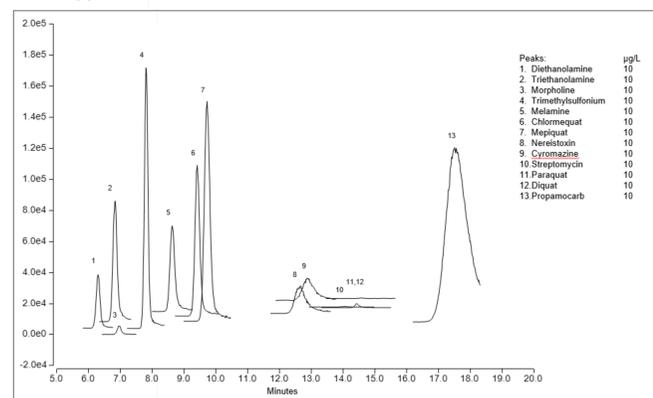
Figure 3: Column : Dionex IonPac CS17 2 x 250 mm. Injection volume: 5 µL. Flow rate: 0.4 mL/min. Eluent: 0 min – 1.0 mM MSA, 4 min – 3.2 mM MSA, 10 min – 15 mM MSA, 14 min – 40 mM MSA. SRM transitions as shown in Table 4.
