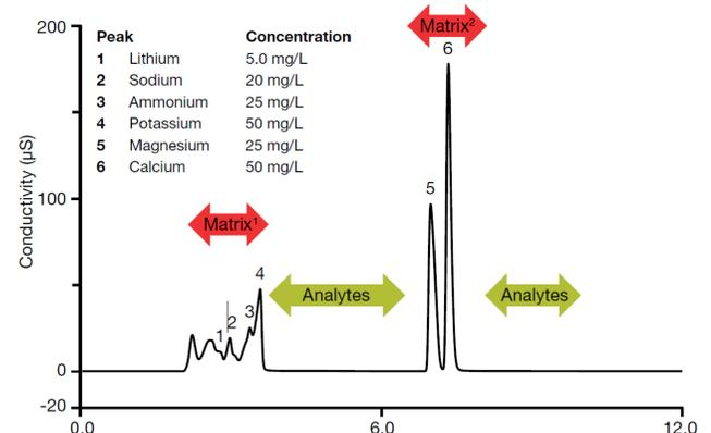
Figure 4: Column : Dionex IonPac CS21-Fast-4µm 2 x 250 mm. Injection volume: 10 µL. Flow rate: 0.3 mL/min. Eluent: 0 min – 3.0 mM MSA, 3.6 min – 3.0 mM MSA, 6.0 min – 22.0 mM MSA, 15 min – 25 mM MSA.
