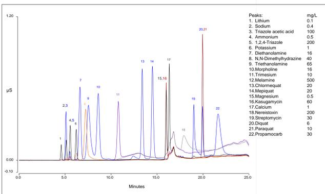
Figure 1: Column : Dionex IonPac CS17 2 x 250 mm. Injection volume: 2 µL. Flow rate: 0.4 mL/min. Eluent: 0 min – 2 mM MSA, 8.5 min – 2 mM MSA, 14.5 min – 10 mM MSA, 20.5 min – 60 mM MSA.
