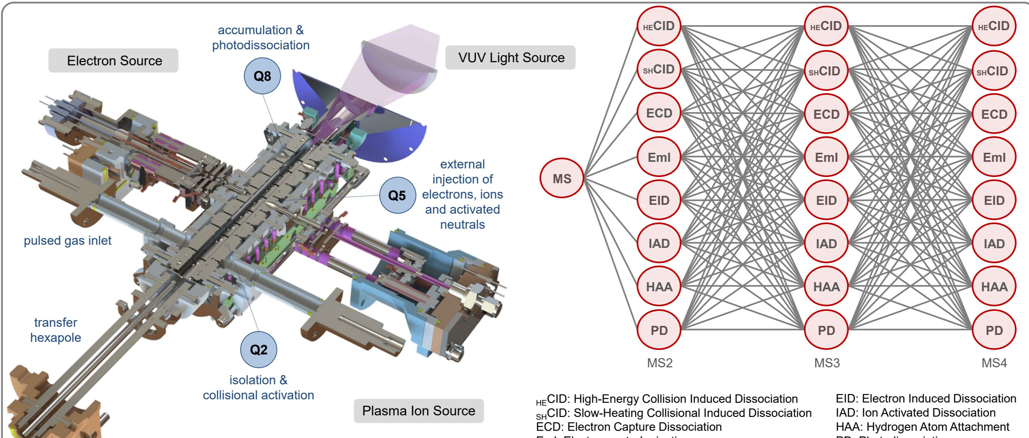
The Omnitrap platform is a segmented RF linear ion trap enabling multidimensional multiple-stage tandem mass spectrometry.
