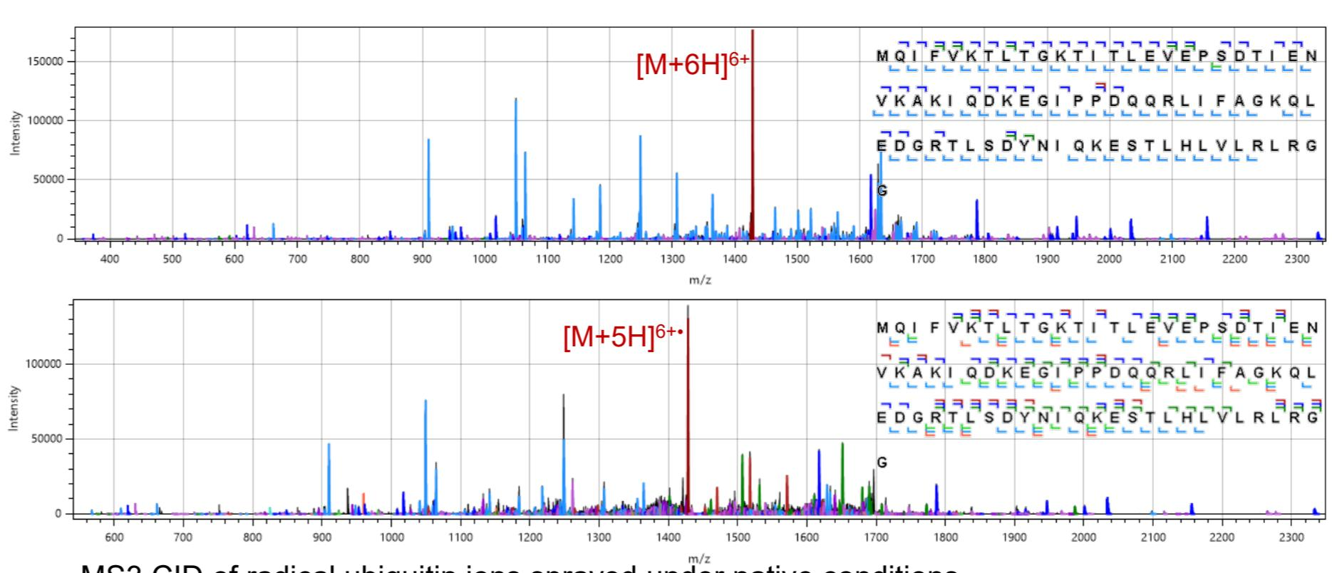
The efficiency of ExD reactions available in the Omnitrap platform are evaluated using a BSA tryptic digest separated in a 25 cm long PepSep C18 column and by operating the Orbitrap MS in DDA mode. EID reactions are performed within a 50 ms time window and ECD reactions within 80 ms. Examples of MS2 EID and MS2 ECD spectra demonstrate enhanced sequence coverage and complementarity for all peptides independent of charge state. Results are compared with HCD fragmentation.
