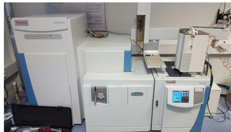
Multi-Shot Pyrolyzer (Frontier EGA/PY-3030D) with Auto-Shot Sampler (AS-1020E) coupled to an Exactive GC Orbitrap mass spectrometer
