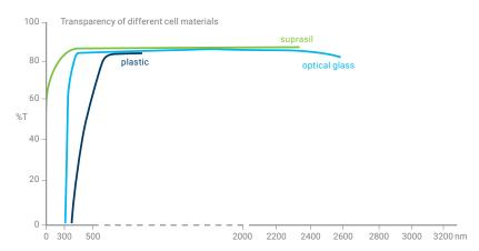
Figure 22. Transparency of common optical cell materials.
