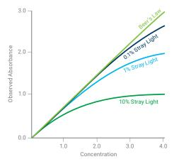
Figure 28. A UV-Vis system with poor stray light performance will show deviations from Beer's Law. This makes concentration calculations unreliable.
