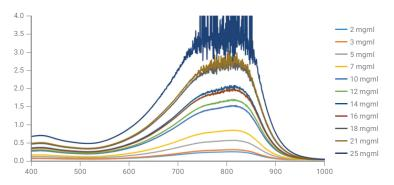
Figure 29. As sample absorbance increases progressively less light reaches the detector. This increases noise in the results and an obvious spiky signal will be observed in scanning mode.
