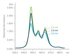
Figure 25. Overlaid scans, each measured using a different instrument slit.
