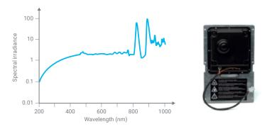
Figure 11. Intensity spectrum of the Xenon lamp.
