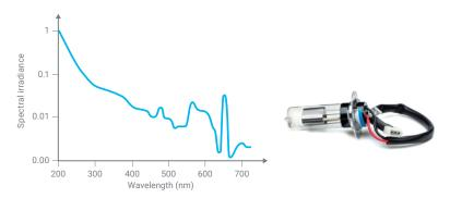
Figure 9. Intensity spectrum of the deuterium arc lamp.
