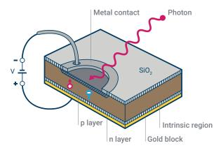
Figure 18. A silicon photodiode detector.
