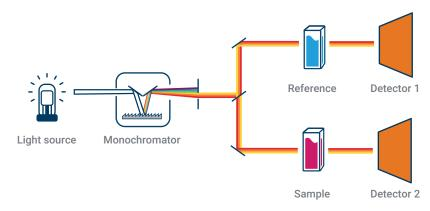
Figure 16. Schematic diagram of double beam optical system, with dual detectors.
