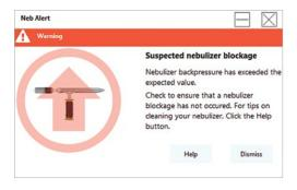
The Neb Alert function of the Agilent 5800 and 5900 ICP-OES alerts the analyst when the nebulizer back pressure changes—indicating either a blockage or a leak.
