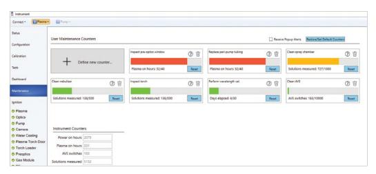
Both the Agilent 5800 and 5900 ICP-OES instruments include the early maintenance feedback function. This function counts the number of samples measured. It displays screen alerts, reminding the analyst to perform cleaning and maintenance functions, after the nominated number of samples have been measured.
