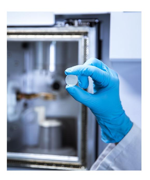
Analysts should include the cleaning of pre-optic windows in the regular maintenance schedule for an instrument. Running the automated instrument performance tests each day will uncover any loss in instrument sensitivity.
