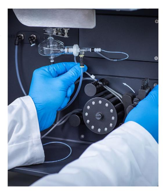
Regular routine maintenance prevents the occurrence of peristaltic pump tube problems. Checking the tube's elasticity, roundness, connection, and tension at the start of each day, or after a certain number of samples, is important. These checks can reduce the risk of having to remeasure samples due to pump tubing problems.
