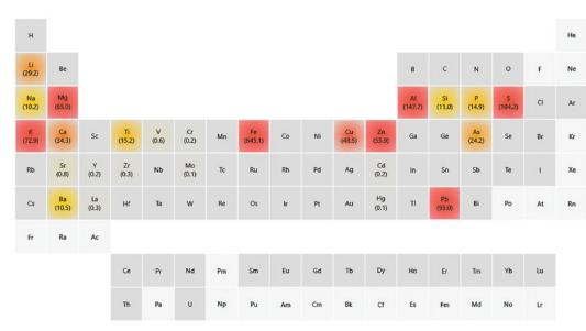
The Agilent IntelliQuant function semi-quantifies up to 70 elements in a sample. This is useful when developing a new method or measuring unknown samples from a new source.
