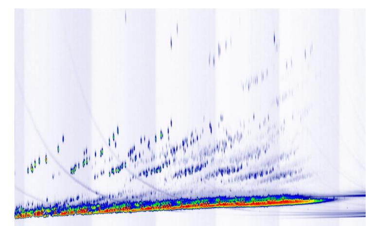
GC X GC Raw Linear Plot Chromatogram: 1 Minute of Run Time Showing 10 Modulation Cycles. Each Peak has a width of approx. 300ms at the base.
