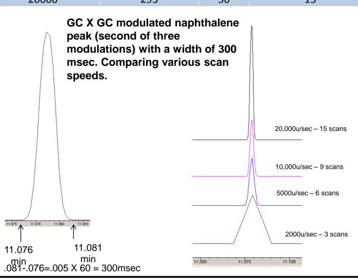
Data acquisition of 300msec peaks is very demanding. As shown in the above figure, only the 20,000 u/sec scan rate resulted in enough scans to fully characterize the modulated peak appears to be about twice as wide and much shorter than the others. Below is a section of a FAMES GC X GC plot that shows the difference in resolution due to data point
