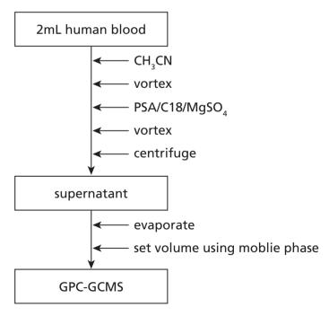
Figure 1 Schematic flow diagram of the sample preparation
