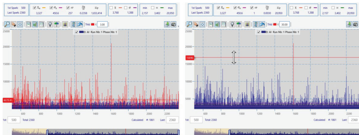
Two single Chart views of the same analysis run of sample CKD 182A with peak detection thresholds at 3\sigma (left) and 30\sigma (right) above background signal. The values of the key parameters are interactively recalculated when manually sliding the peak detection threshold up or down.
