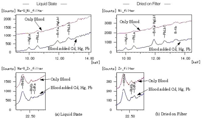
"Only Blood" Profile has offset (Backgrounds are same between "Only Blood" and "Blood added Cd, Hg, Pb ") Figure 1: Qualitative Analysis of Cd, Hg, Pb 10ppm in Blood
