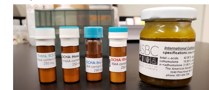
Figure 4- Set of humulone standards use for compound confirmation.
