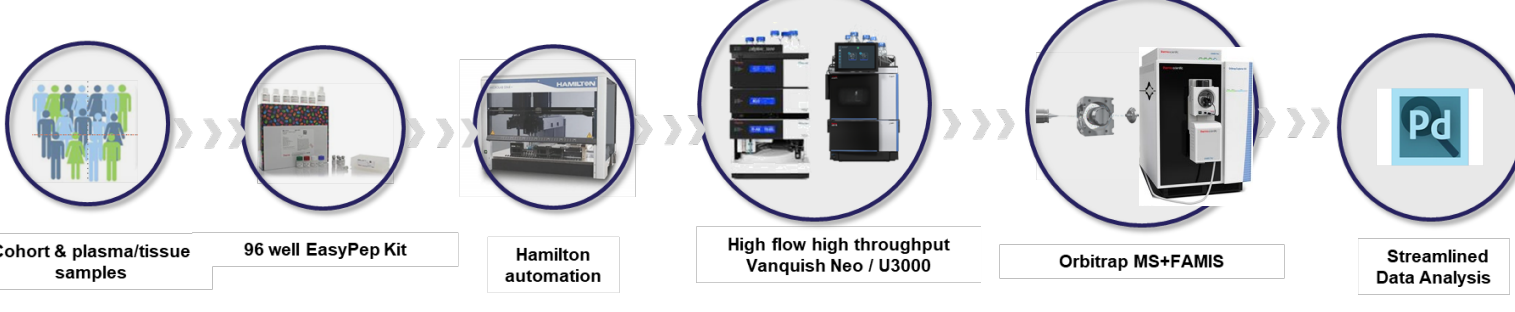
Figure 2. High throughput plasma workflow including a Vanquish Neo UHPLC/U3000 system and Orbitrap Exploris 480 mass spectrometer coupled with FAIMS Pro Interface.
