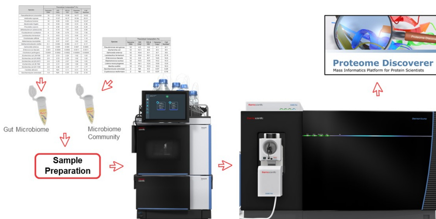
Figure 1. Deep metaproteomic workflow including a Vanquish Neo UHPLC system and an Eclipse Tribrid mass spectrometer coupled with FAIMS Pro Interface.
