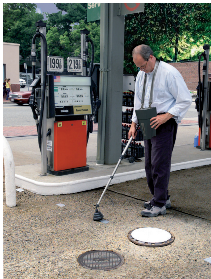
This probe assists the operator when checking underground objects or objects out of arms reach. The tip has a small funnel to better convey helium to the probe.
