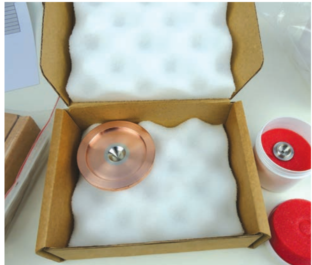
Figure 9. The sampling cone is loosely packed into the foam insert of the cardboard package used by Competitors I and S, which means the cone may be damaged with rough handling.
