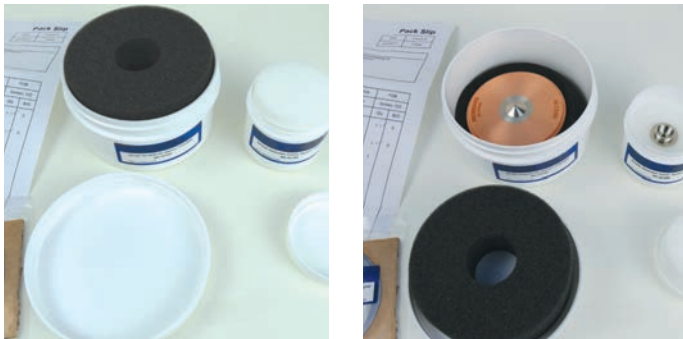
Figure 8. Packaging used for Competitor E's sampling (lower left) and skimmer (lower right) cones, based on a cylindrical plastic container.
