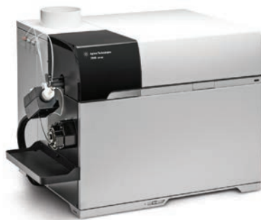
Figure 5. An Agilent 7900 single quadrupole ICP-MS system was used for performance testing of the sampling and skimmer cones.
