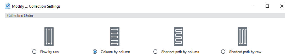
Figure 3. Fraction collection orders available with the open-bed fraction collector. The column by column mode proceeds from left-to-right and front-to-back.
