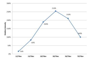
Figure 3. Comparing sensitivity at different electron energies (eV): x-axis is the lower electron energies compared to 70 eV; y-axis is the relative intensity of the sum of all target ions for 111 doping analytes in positive QC at 1/2 MRPL.
