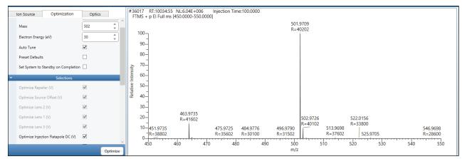
Figure 1. Orbitrap Exploris GC tune VeV window. The eV and tune mass can be selected by the user prior to tuning that takes < 1 minute.
