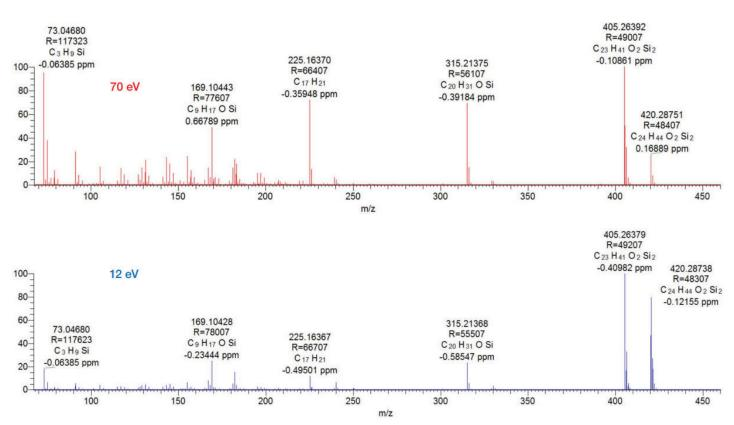
Figure 2. Comparison of 19-NA mass spectra acquired using VeV, at 70 eV and 12 eV. There is reduction in fragmentation at the lower end and enhancement of the molecular ion when using 12 eV.
