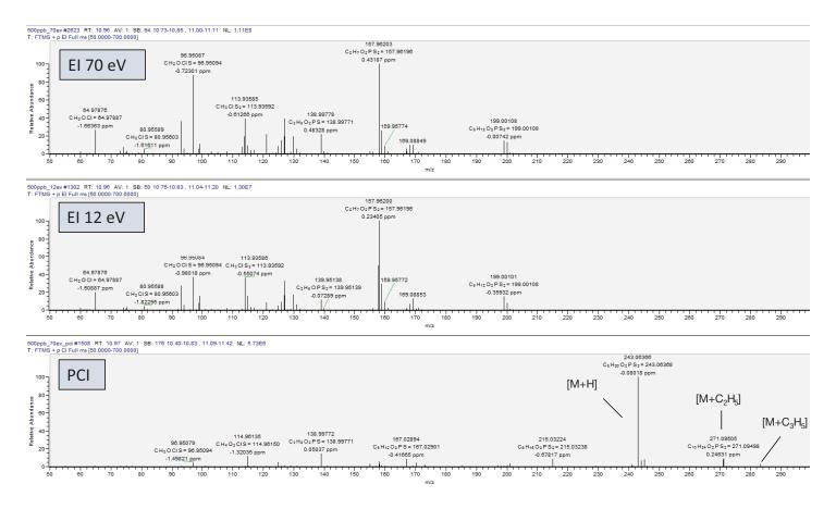
Figure 6. Spectra obtained for the compound ethoprophos at EI 70 eV (upper), 12 eV (middle), and chemical ionization (lower)
