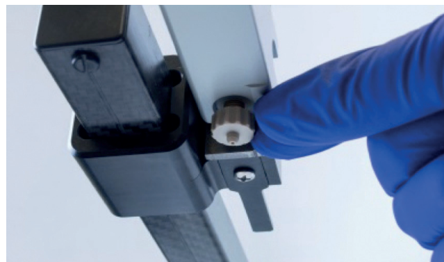
Figure 4. Displayed is the 1.0 mm drop-former delivered with the Fraction Collector F. There are two drop-former configurations: 0.4 mm drop-former with corresponding diverter valve and 1.0 mm drop-former with corresponding diverter valve.
