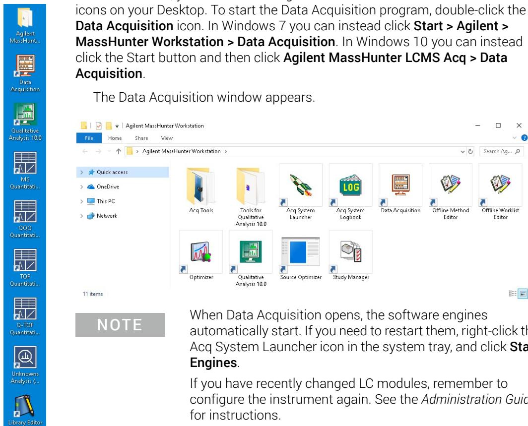
When Data Acquisition opens, the software engines automatically start. If you need to restart them, right-click the Acq System Launcher icon in the system tray, and click **Start Engines**.
