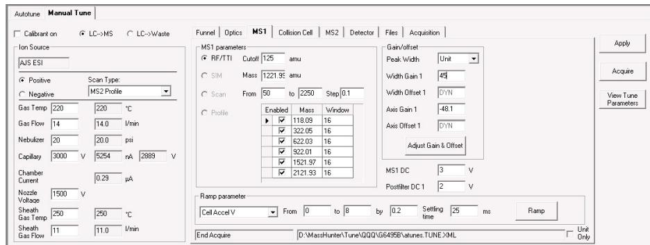
c If the failure occurred in MS2, click the **MS2** tab. Select the **Peak Width** based on which resolution failed in Checktune. Then, click **Adjust Gain & Offset**.
