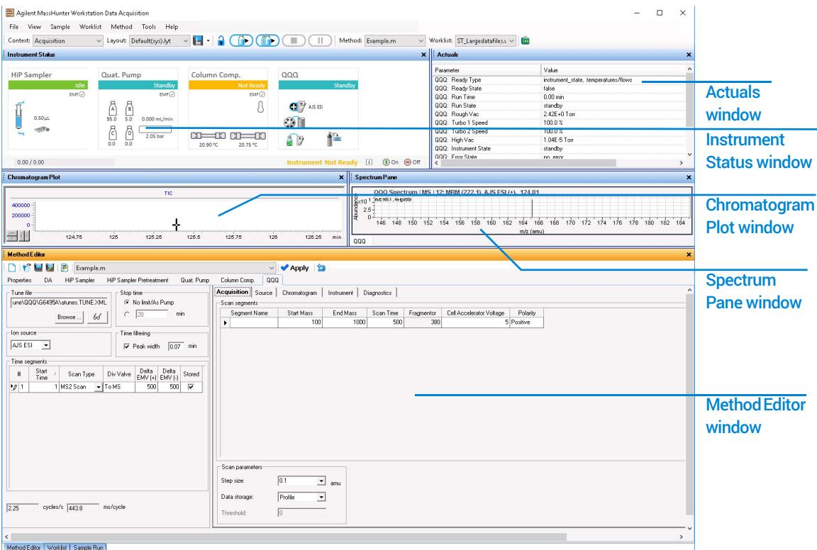
**Figure 1.** Main window of the Data Acquisition software program. The Sample Run and Worklist windows are tabs grouped together here. These three windows are “sharing” this space. You click the tab to switch to a different window.
