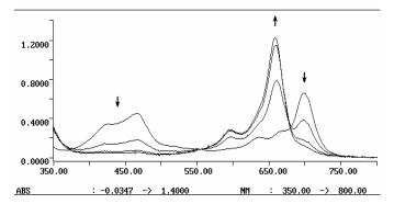
Figure 3. Spectral changes that occur upon the addition of  $CO_2$  to Co(I)Pc in 0.1M (TBA)BF<sub>4</sub>/DMF at a potential of -1.8 V vs SCE
