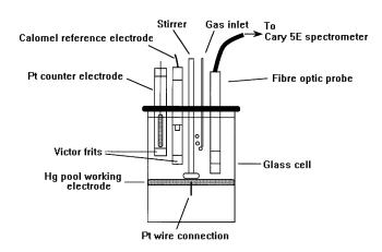
Figure 1.Design of the electrochemical cell used for spectroelectrochemical experiments with a fiber optic probe
