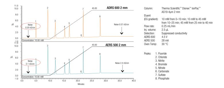
Figure 4. Comparison of baseline noise on a system running a potassium hydroxide gradient using constant current (Dionex AERS 500 Anion Electrolytically Regenerated Suppressor) and dynamically regenerated (Thermo Scientific<sup>™</sup> Dionex<sup>™</sup> ADRS 600 Anion Dynamically Regenerated Suppressor) suppressors.
