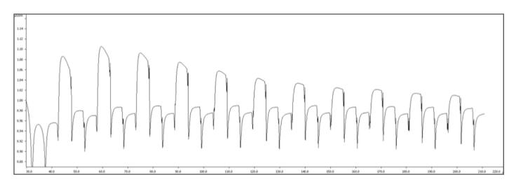
Figure 2. Example of baseline disruptions resulting from automatically switching packed bed suppressors. If standards are run on different suppressor cartridges from samples, spurious results may be obtained.
