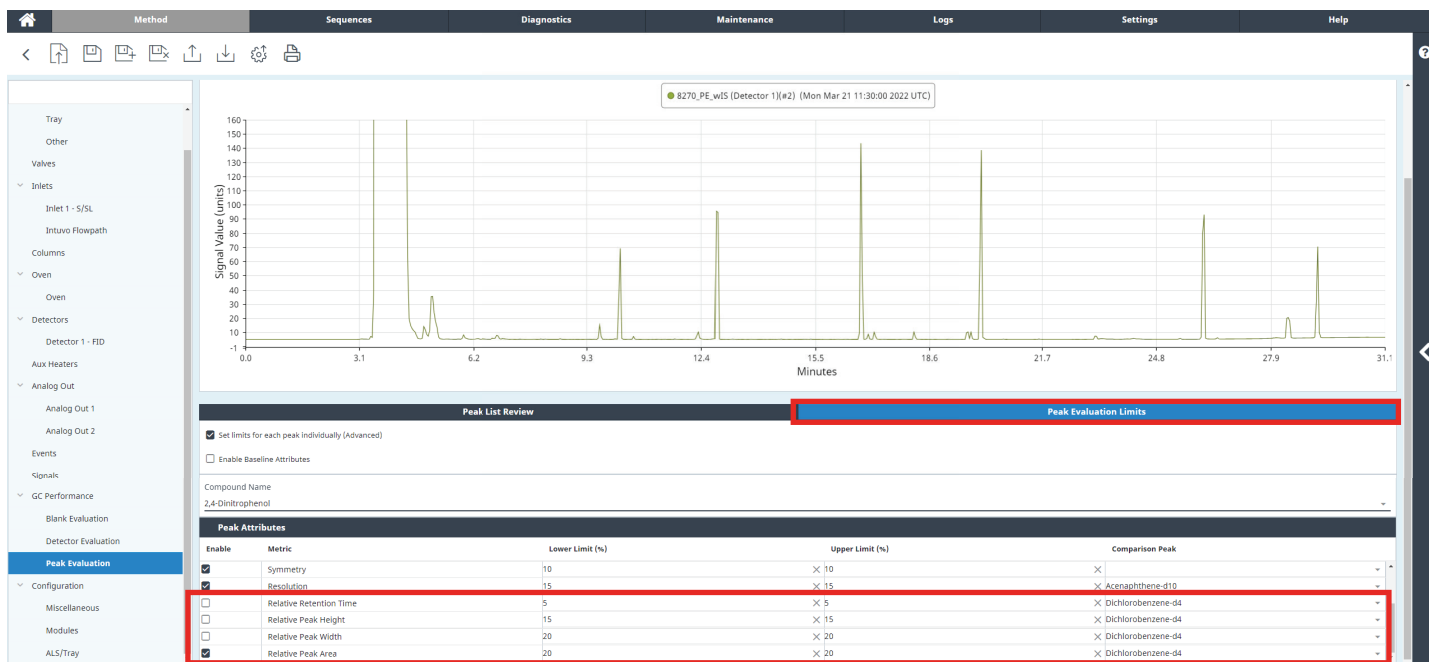
Figure 26. Within the Peak Evaluation Limits tab, selecting the Set limits for each peak individually (Advanced) check box and selecting relative parameters to be monitored.
