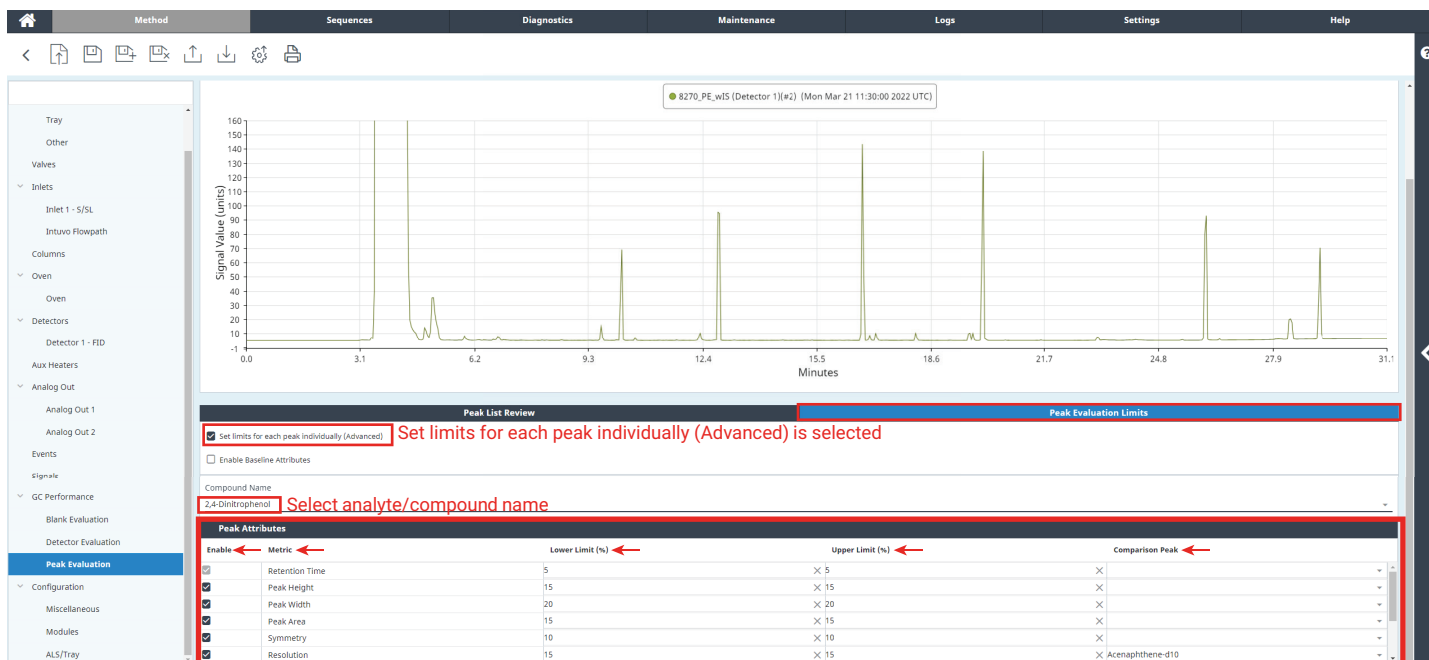
Figure 25. Within the Peak Evaluation Limits tab, selecting the Set limits for each peak individually (Advanced) check box and selecting an analyte.
