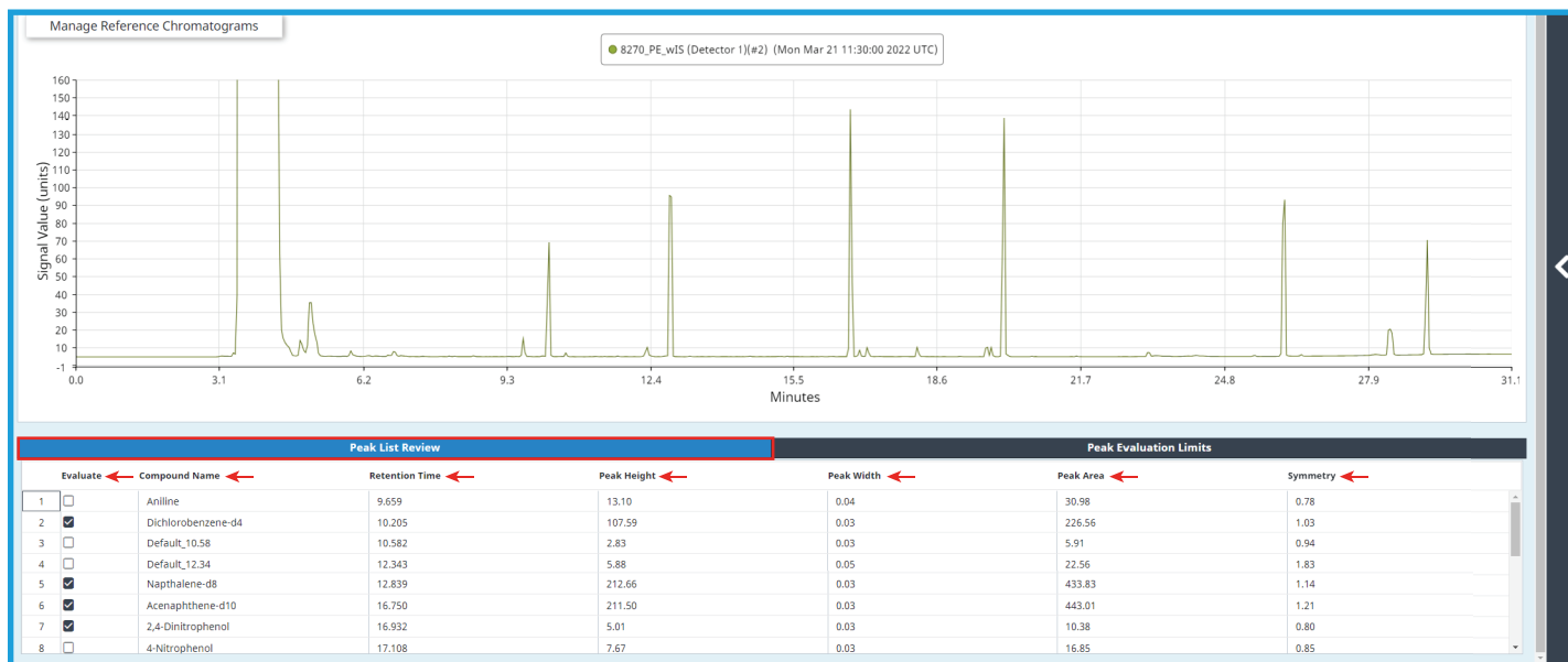
Figure 21. Peak List Review tab showing the parameters that can be evaluated from within Peak Evaluation.
