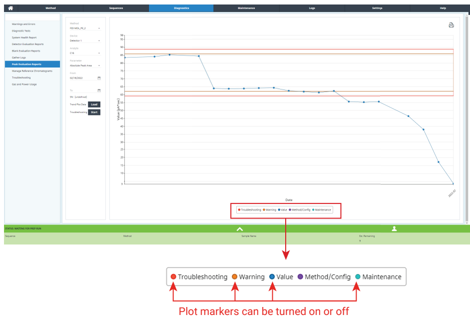
Figure 22. Peak Evaluation Trend Plot markers, which can be turned on or off.
