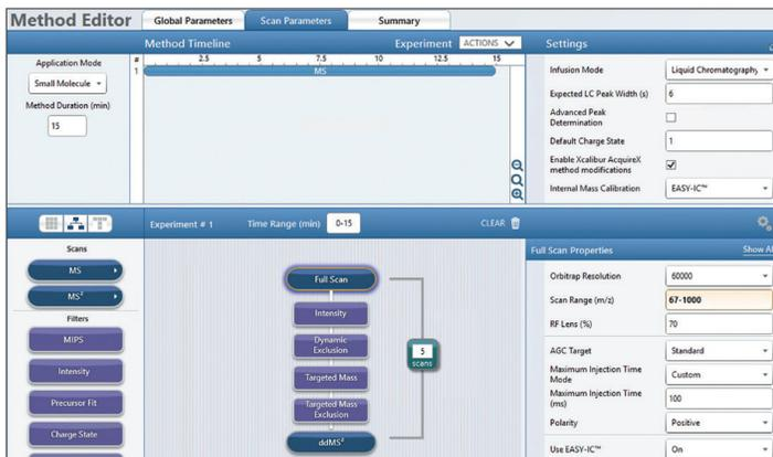
Figure 2. Ease of use: Screenshot of the method editor window to setup the mass spectrometer parameters. Plug-and-play nodes enable you to easily set and customize the analysis to maximize data quality and instrument performance.
